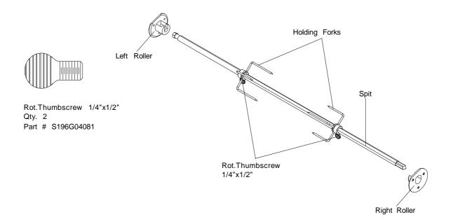
5. Insert the right side of the assembled Rotisserie Spit into the Right Roller and Motor Transmission. Next insert the left side of the Spit into the Left Roller (See diagram below.)
