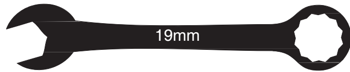
19mm Spanner (wrench) for Gas Inlet Connection
