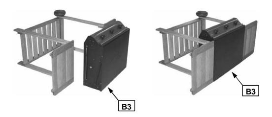
Lay the assembled trolley on its side. Lay the body (B3) on its back and slide into position between the trolley legs. **Warning:** Care must be taken to ensure lid does not fall open unexpectedly.
