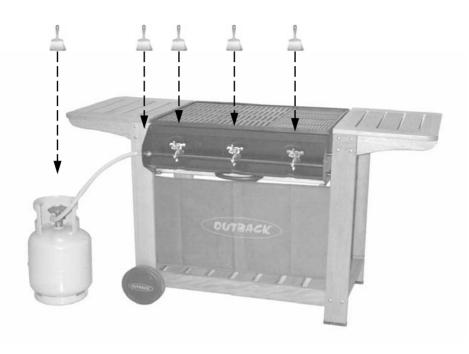
**11a.** Connect the gas hose (B2) to the barbecue (Before the Leak Test). Ensure the mating faces of the connection are clean and not damaged. Do not use any sealing tape, paste, or liquid on the joint. The nut must be tightened with the use of a spanner. Do not use force which may damage the assembly.
