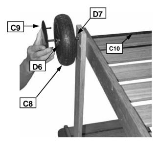
Turn the trolley over so that it stands on its side shelves. Slide the axle (C10) through the corresponding holes in the short legs. Place a washer (D7) on each end of the axle. Slide the wheels (C8) over each end of the axle. Secure the wheels into place with the locknuts (D6). Snap the hubcaps (C9) into the wheels.
