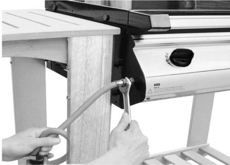
Connect the hose and regulator (B12) to the BBQ. Ensure the mating faces of the connection are clean and not damaged. Do not use any sealing tape, paste or liquid on the joint. The nut must be tightened with a spanner. Do not use force which may damage the assembly.
