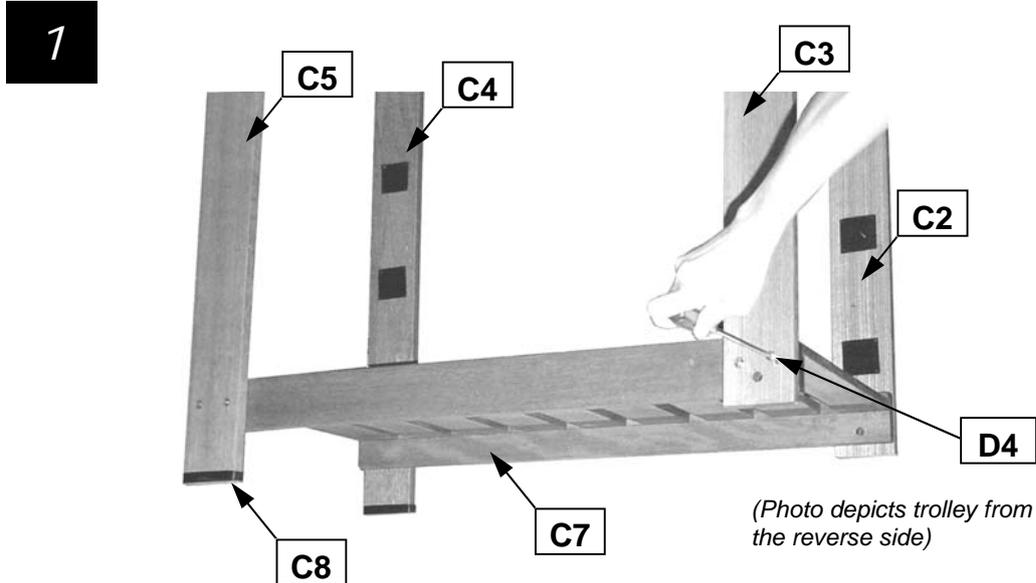
Attach the short (C2,C3) and long legs (C4,C5) to the trolley base (C7) using the 1/4-20UNC bolts (D4). Take care to fix the legs with Velcro attached as shown in the illustration.
