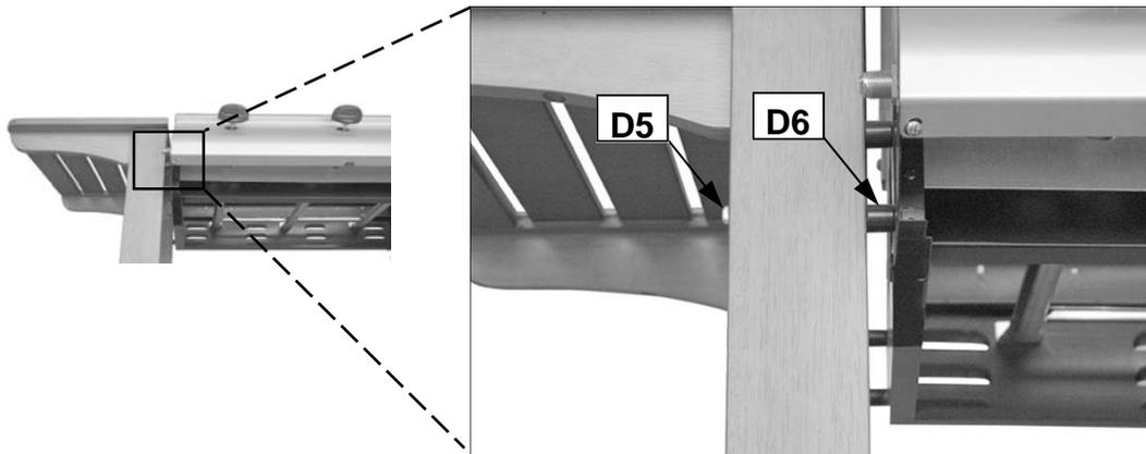
With the barbecue laid on the ground, insert a M6x95 bolt (D5) through the short leg, through a spacer (D6), and secure the bolt into the sidewall of the body. Repeat the process for all the legs until the body is completely fixed to the trolley.
