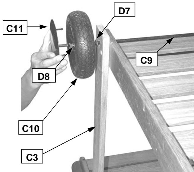
Turn the trolley over so that it stands on its side shelves. Slide the axle (C9) through the corresponding holes in the short legs (C2,C3). Place a washer (D7) on each end of the axle. Slide the wheels (C10) over each end of the axle. Secure the wheels into place with the locknuts (D8). Snap the hubcaps (C11) into the wheels.
