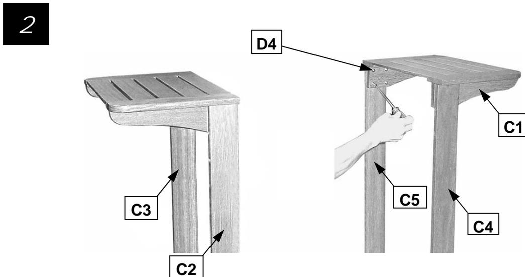
Attach the side shelves (C1) to the short (C2,C3) and long (C4,C5) legs using the 1/4-20UNC bolts (D4).
