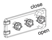
By dialing open the ventilation control knobs, in conjunction with the chimney damper, you allow air to enter the combustion chamber and circulate through the oven which will increase the flames and cause the oven temperature to rise.
