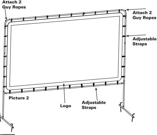
Using the supplied guy wires and stakes secure the frame to prevent it from moving around in windy conditions or tipping over.
